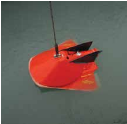
▲ A 150 kHz ADCP used to measure currents housed in a depressor fin. Photo: Dave Janka
